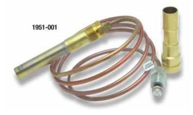
Robertshaw® thermopiles are the industry leader for gas appliance applications. Their primary function is to ensure a standing pilot light is operative so that on a call for heat, the main burner gas will be properly ignited. Thermopiles are placed in gas applications to detect the existence of a flame for safety purposes by shutting off the potential gas flow to a burner.
