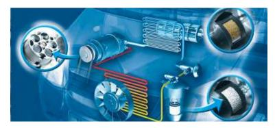
Oil plays an important role in the air-conditioning system, no matter whether it's required when the compressor is replaced or for refilling during the air-conditioning service. Like blood in the human body, the oil fulfills vital tasks in the air-conditioning system.
