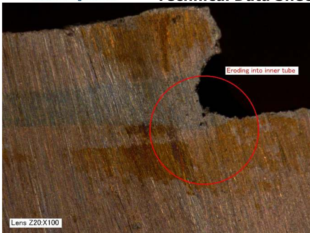
Figure 1: Erosion of Sil-Fos into Copper base metal
