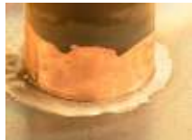
Flux condition near brazing temperature
