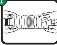
Extend duct to its full length, and position, cut and discard any excess.
