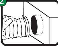
Attach one end of flexible duct to exhaust outlet pipe using clamp (Not Included) and tighten.
