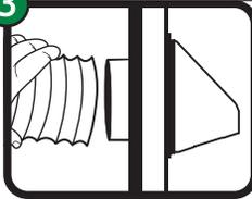
Attach the other end of flexible duct to vent pipe using clamp (Not Included) and tighten.
