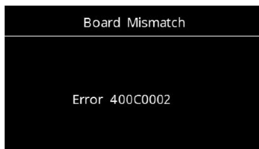
Figure 1: Error code indicating mismatched boards
